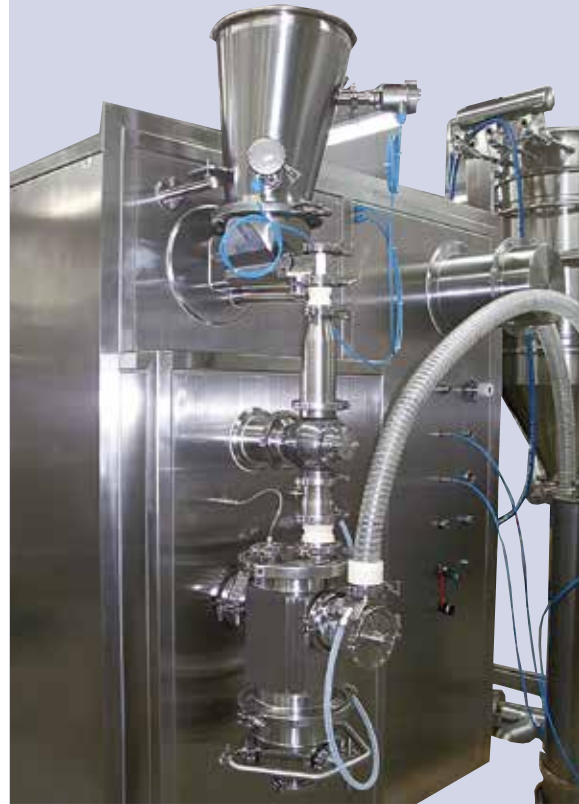
140 AFG - Installation in Reinraumwand
